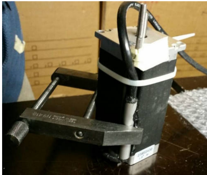
Figure C.4: Clamp the tube in place during curing.
